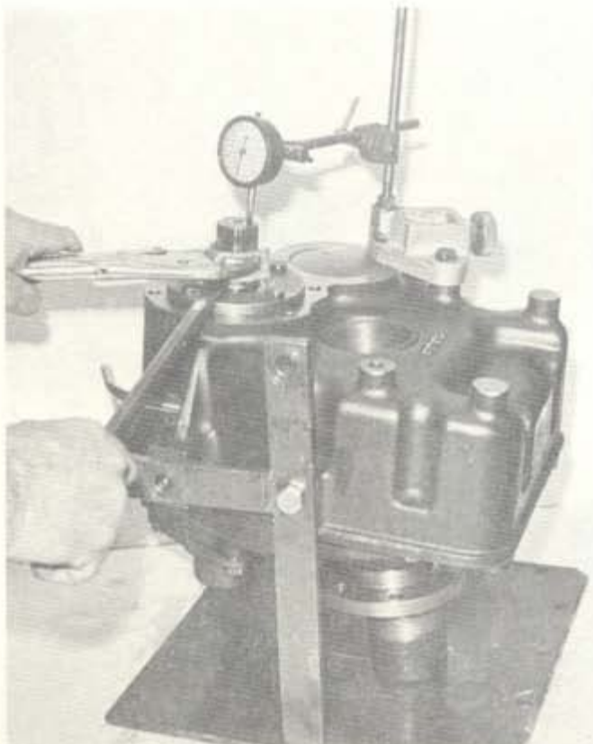
Figure 31. Checking End Play of Forward Clutch Shaft-Upward Pressure Applied.
