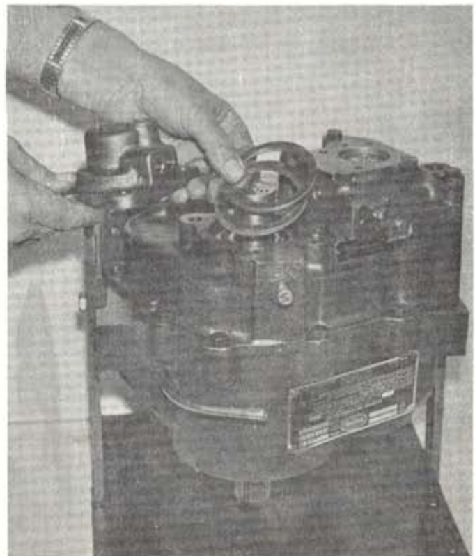
Figure 29. Installing Trial Shim Pack and Collector.
