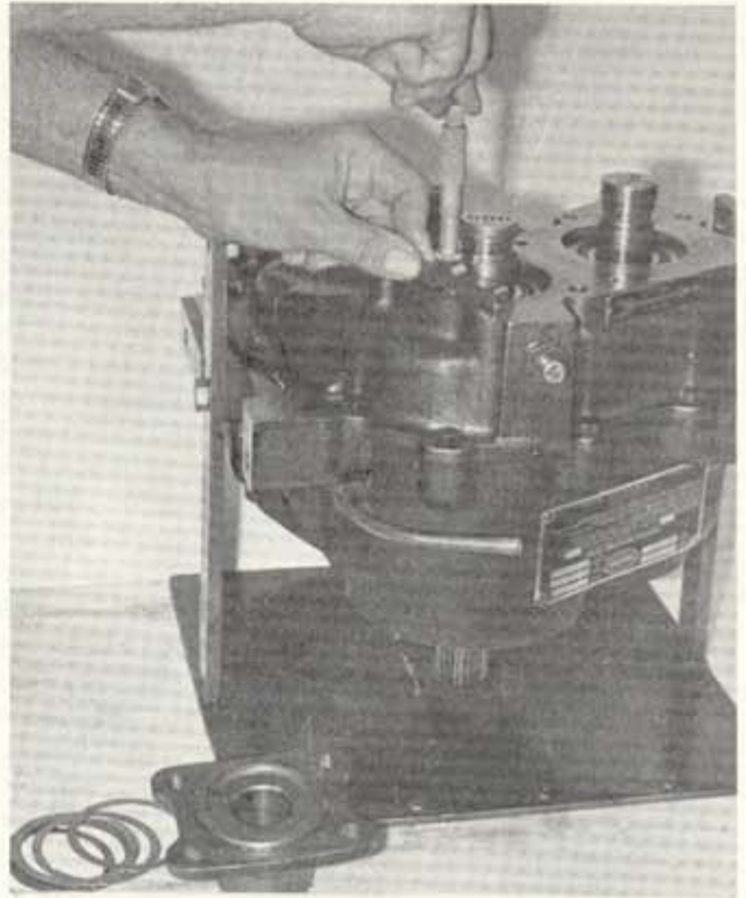
Figure 26. Measuring Rear Cover to Forward Clutch Rear Bearing Cup.
