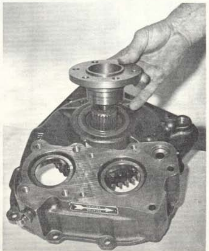
Figure 14. Output Flange Removed.
