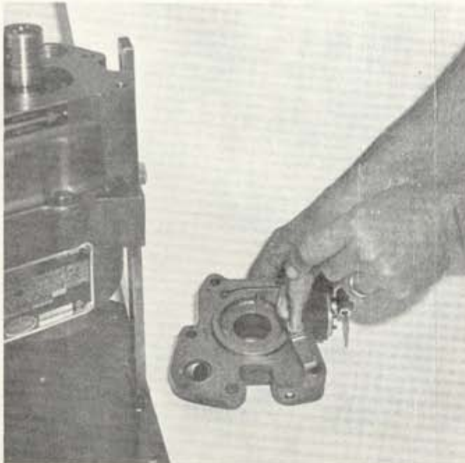
Figure 25. Measuring Valve Body Pilot to Machined Surface.
