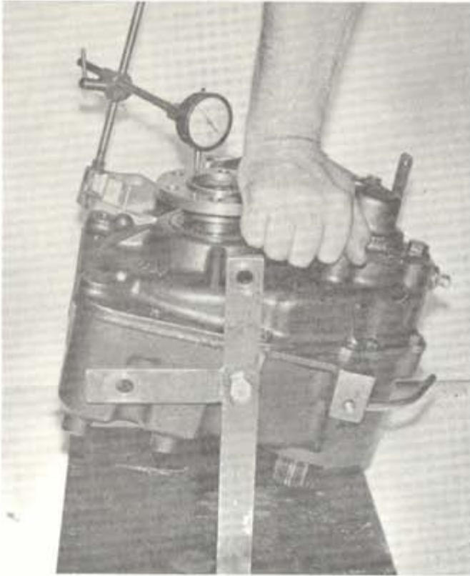
Figure 35. Checking End Play-Downward Force Used.
