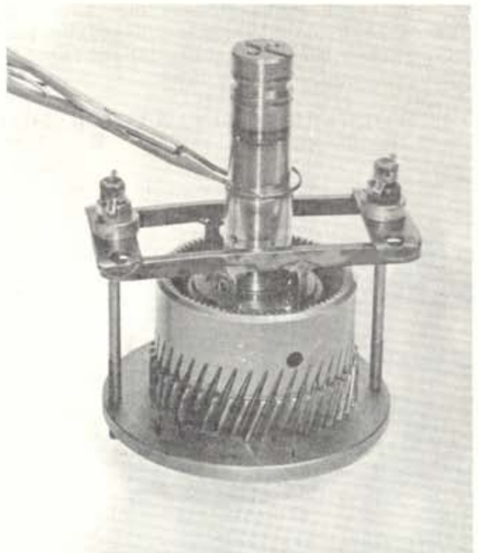
Figure 19. Removing Snap Ring. (Special Tool T-16752).
