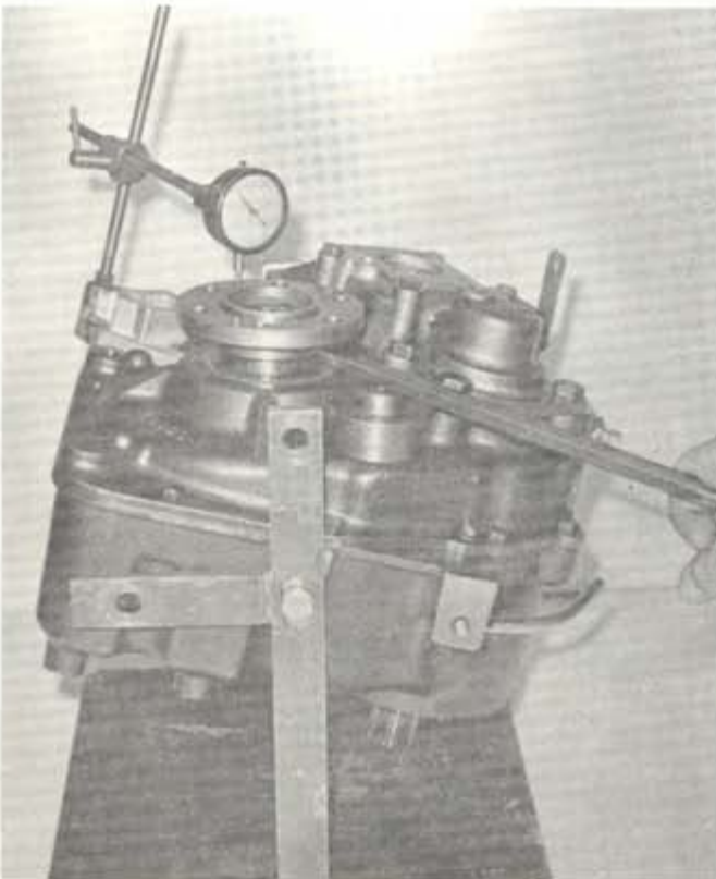
Figure 35. Checking End Play-Downward Force Used.
